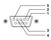
Monitors listed below require RS-232 Null Modem DB9 Cable with male connectors at each end. Depending on the type of Null modem cable, one or two gender changers may be required.
